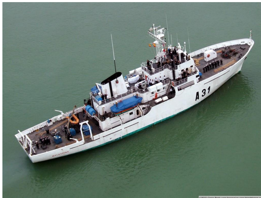
Figure 1. "Malaspina" class oceanic hydrographic vessel.
