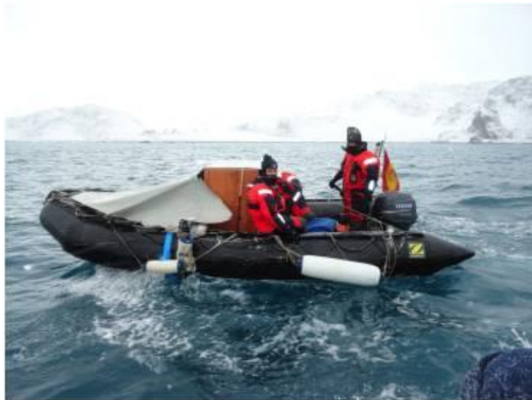
Figure 6. Very shallow water bathymetry system operated from a small rubber boat
